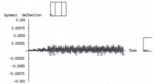
Figure 12. Time history at central point for k_f=7.5 \times 10^8 \text{ N/m}^3 , \gamma=0\% , \omega=50 \text{ rad/s} .
