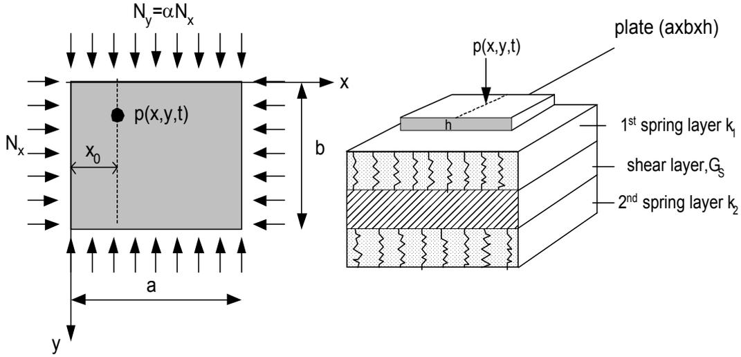
Figure 1. Rectangular orthotropic plate subjected to the bi-axial in-plane loads and dynamic transverse loads supported by a Kerr foundation.
