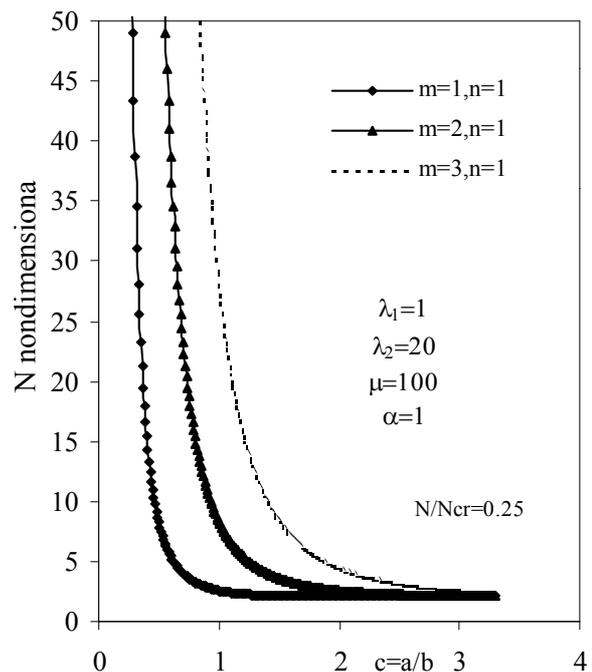
Fig 3. Plate with all edges simply supported and compressed uniformly in both x and y directions.
