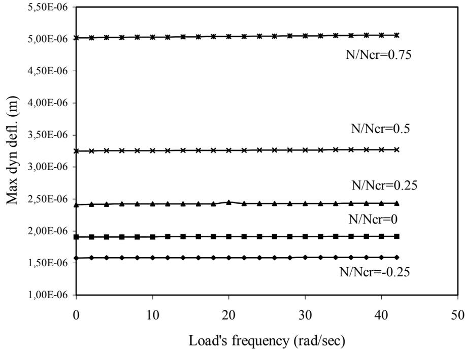
Figure 5. Total dynamic deflection response spectra an orthotropic plate on a Kerr foundation subjected to the dynamic moving load.
