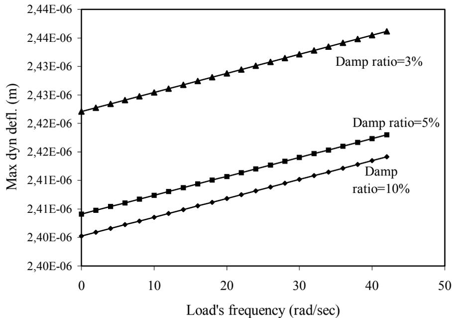
Figure 4. Total maximum deflection response spectra of orthotropic plate on a Kerr foundation subjected to the dynamic moving load.
