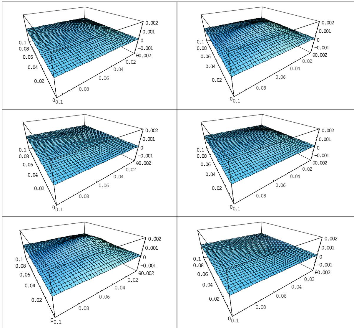
Figure 6. The mode shapes of a plate simply supported on all sides due to dynamic moving load.
