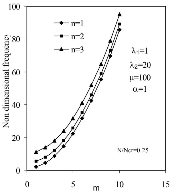
Fig 2. Frequency parameters of the plate with all edges simply supported.
