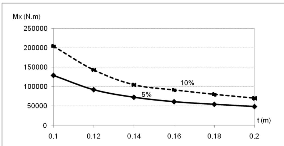
Figure 3. Maximum absolute value of  $M_x$  along the x axes as the function of the thickness.
