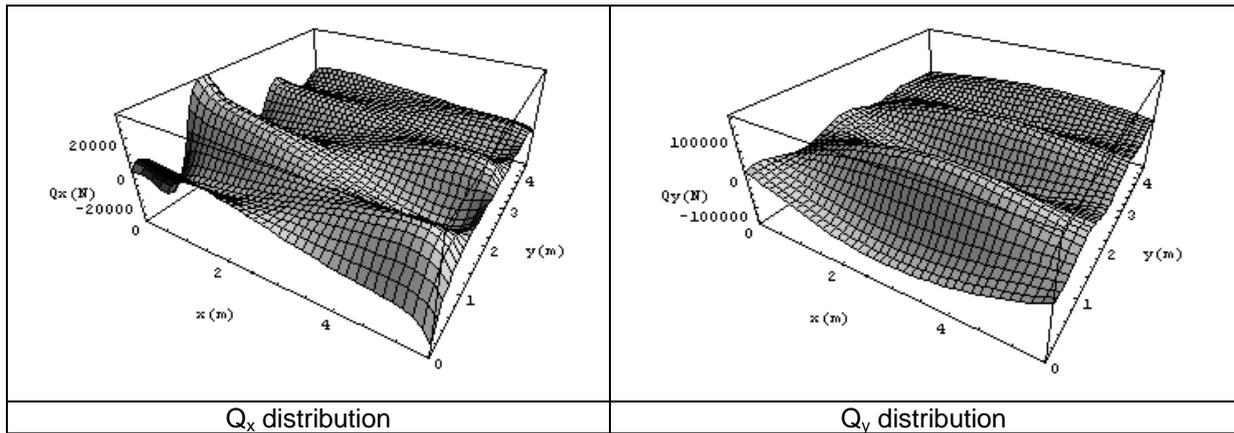
Figure 5.  $Q_x$  and  $Q_y$  distribution along x axes and y axes for model 1 subjected to a localized blast load,  $\gamma=10\%$ ,  $t_d=2$  ms.
