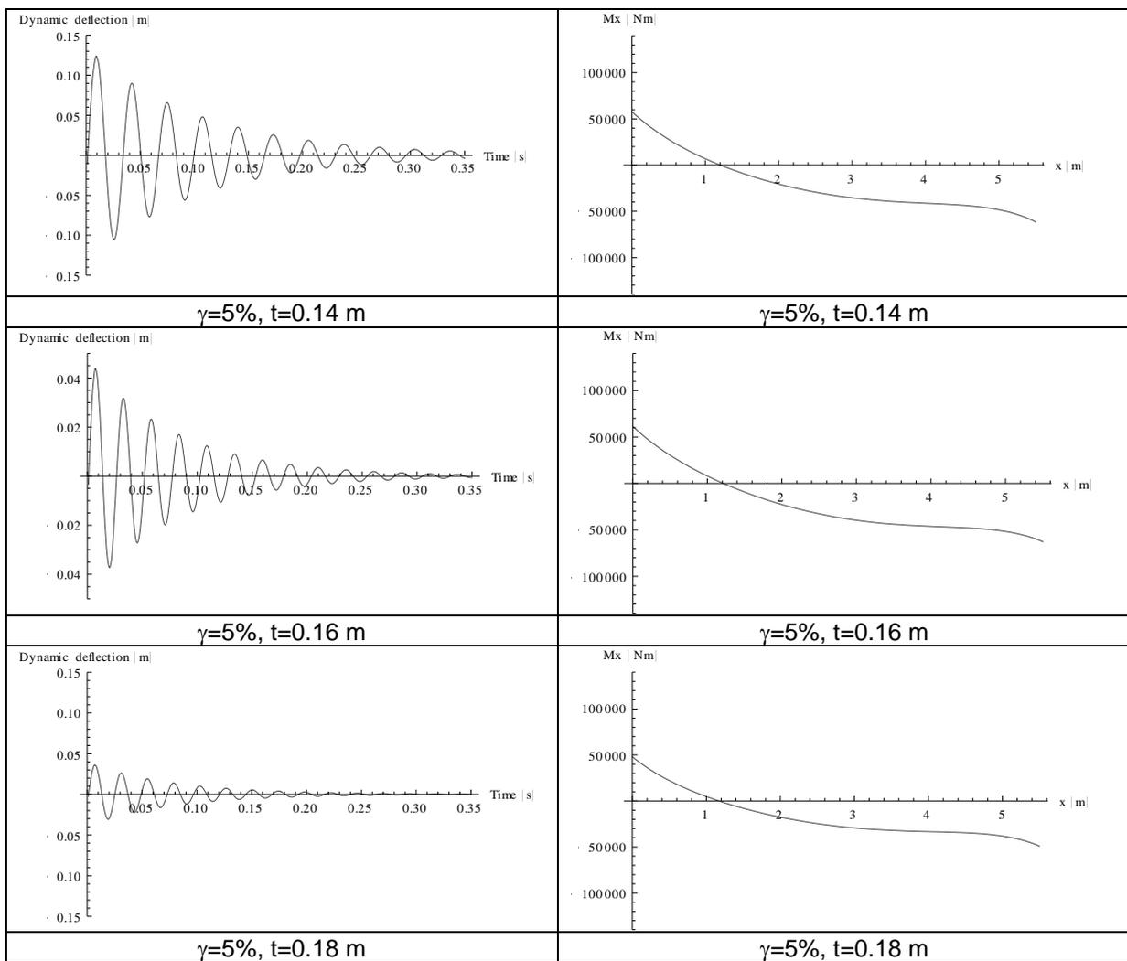
Figure 4. Dynamic deflection time history at the mid-point and moment-x ( $M_x$ ) distribution along x axes for model 1 subjected to a localized blast load.
