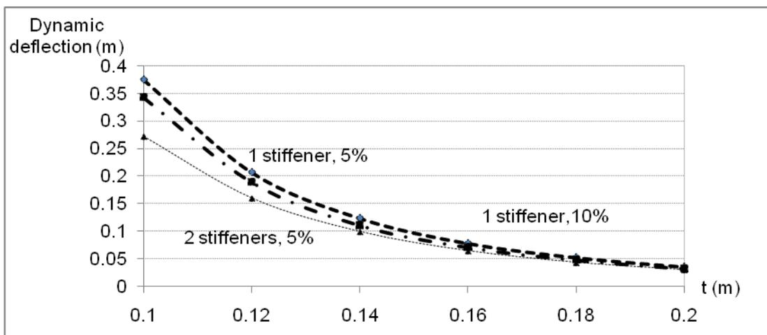
Figure 2. The maximum dynamic deflection at the mid-point of the orthotropic floor plate subjected to a localized blast load for different value of thickness.
