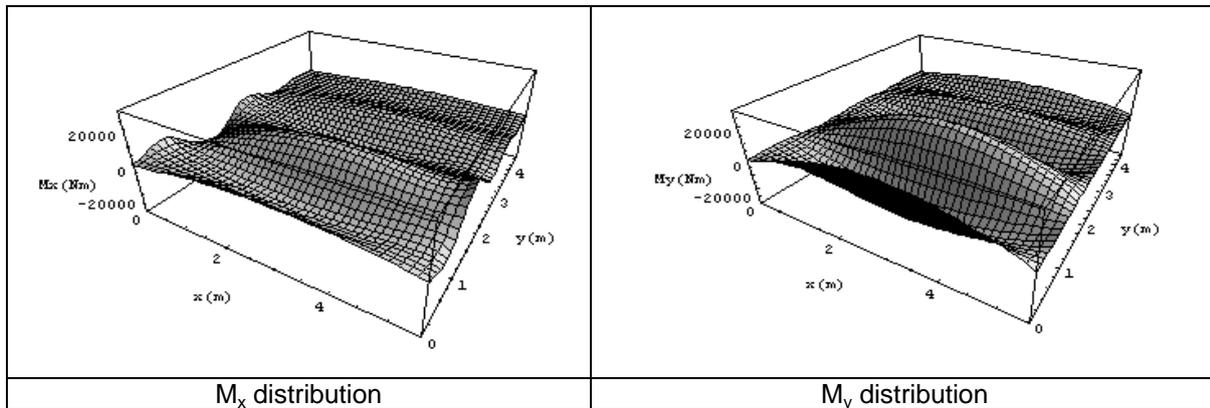
Figure 6.  $M_x$  and  $M_y$  distribution along x axes and y axes for model 1 subjected to a localized blast load,  $\gamma=10\%$ ,  $t_d=2$  ms.
