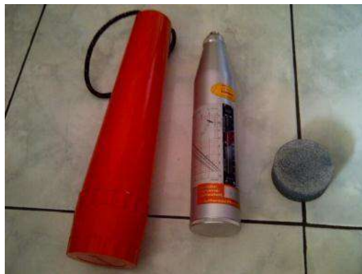
Gambar 4. Schmidt Hammer Test
