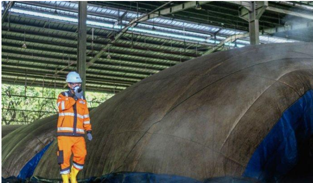
Gambar 3. 10 Biodrying with geotextile
