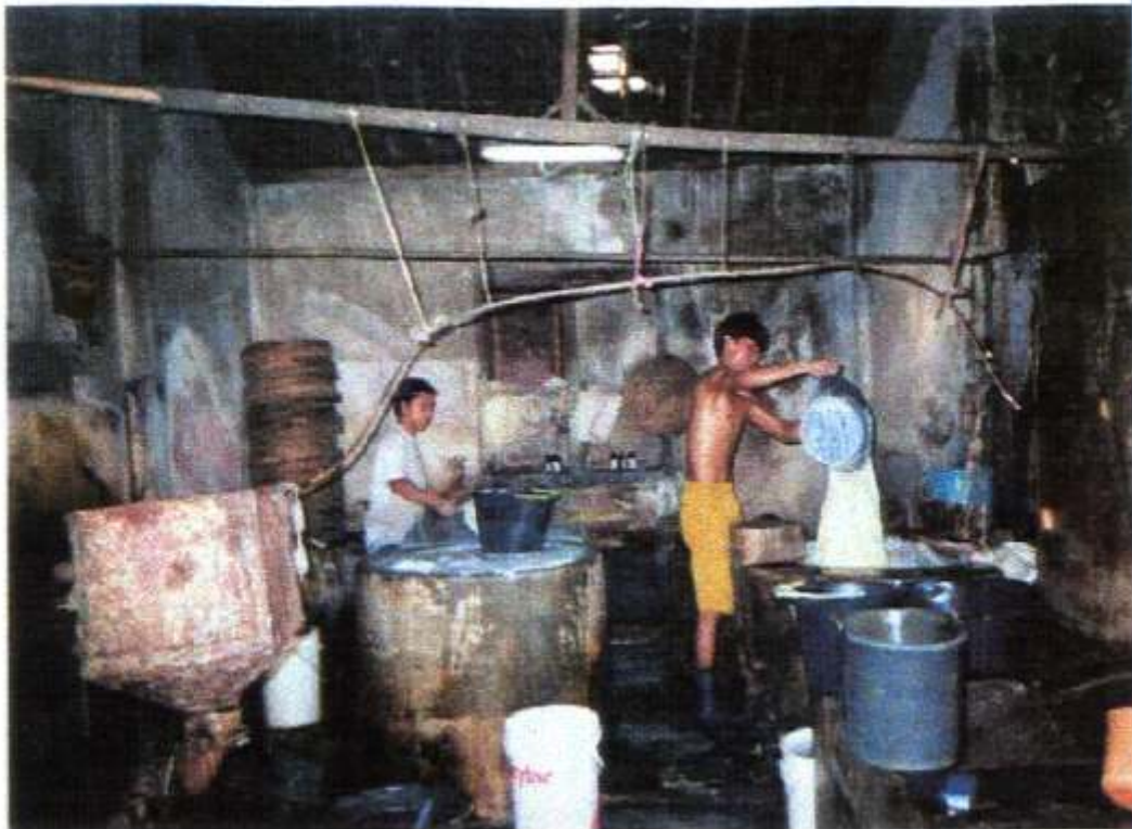
Filtering the Soybean Essence for Curd Formation (Tofu Industries)
